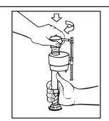
• Replace TOP by engaging lugs and rotating 1/8 turn clockwise. MAKE CERTAIN TIP IS TURNED TO THE LOCKED POSITION. VALVE MAY NOT TURN ON IF TOP IS NOT FULLY TURNED TO THE LOCKED POSITION.
